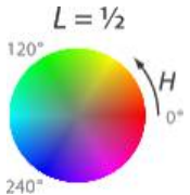
Figure 2: Cross section (at lightness = 0.5) (Those who are using a printed copy of the statement may not see the actual colour, but you will surely notice the change of grey shade)
